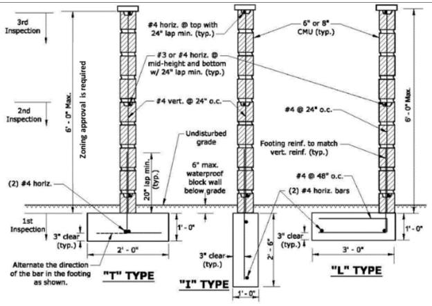
NOTE: IF USING 6" SLUMP STONE BLOCK, IT SHALL HAVE FULL WIDTH INTERIOR CELL DIMENSIONS.
